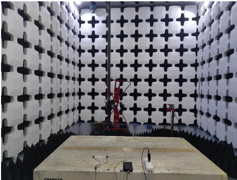
2. Radiated Emissions (Part 15B, Video Player,1GHz-18GHz)
