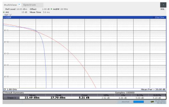
Channel 9538- Peak-To-Average Power Ratio(PAPR)-16QAM
