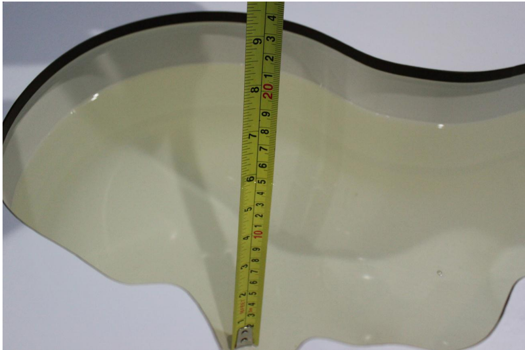
Picture 7-7: Liquid depth in the Head Phantom(5GHz)
