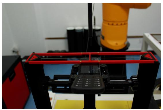
Picture 2: EUT Positioning for RF/T-coil
