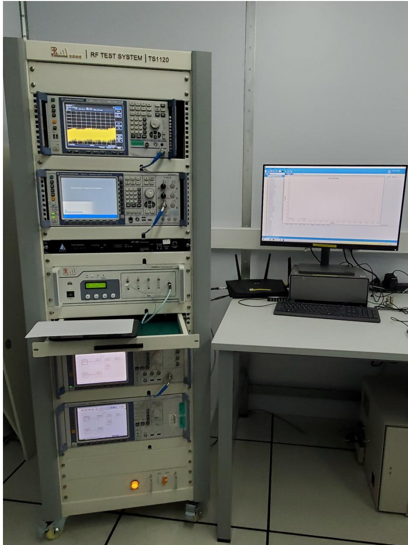
BT/WIFI RF Conducted Test-setup
