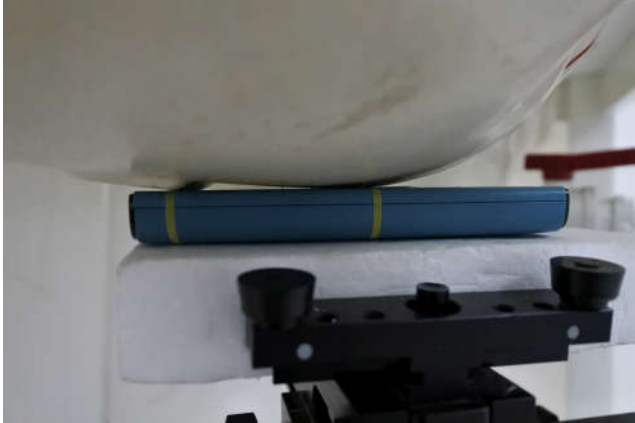
Right Cheek, Test Separation 0 mm
