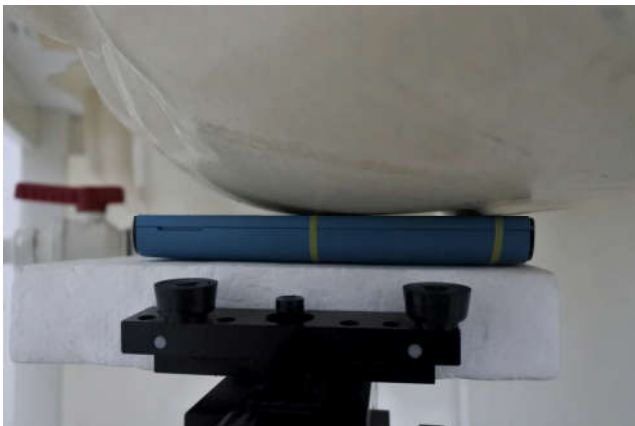
Left Cheek, Test Separation 0 mm
