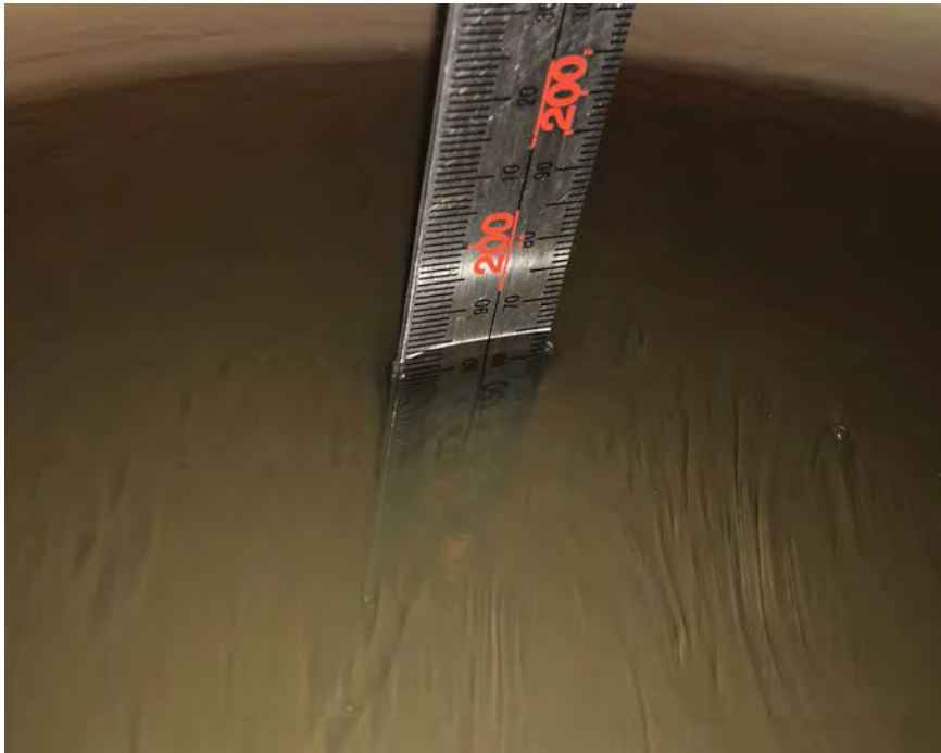
Liquid depth for SAR Measurement
