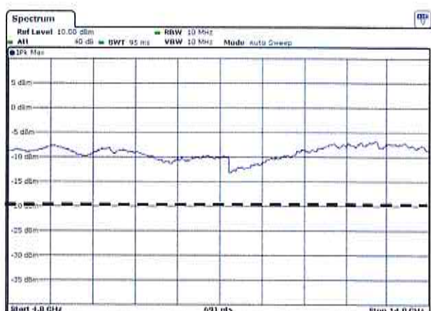
Fig. 2: Output power (high range): > -20 dBm
