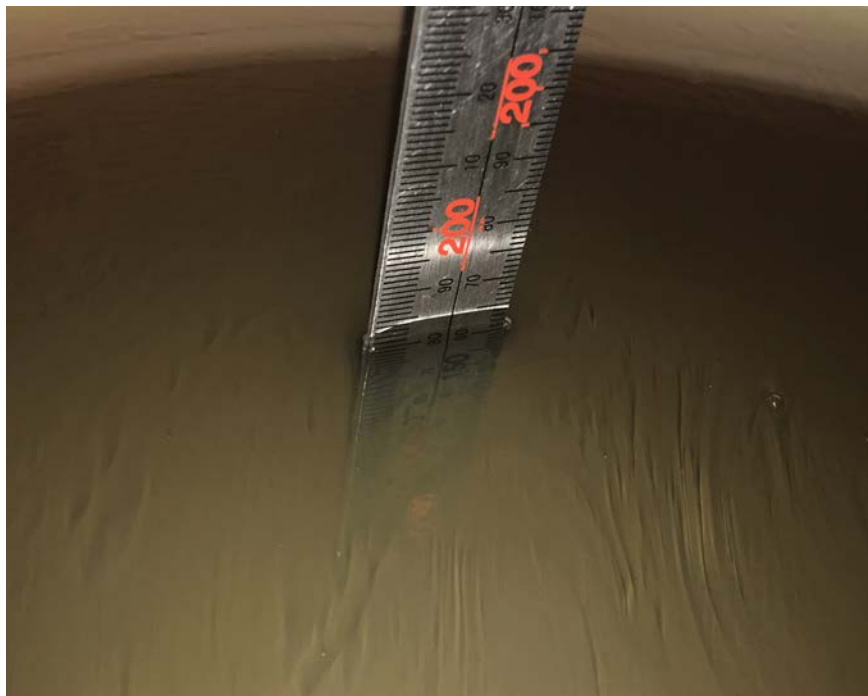
Liquid depth for SAR Measurement
