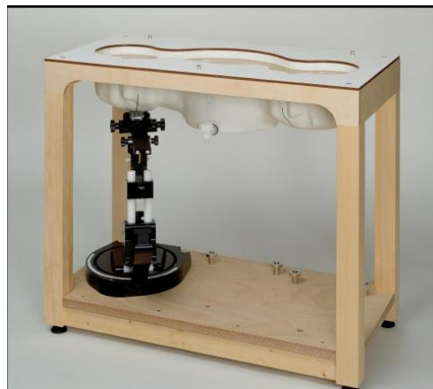
Picture C.8: SAM Twin Phantom
