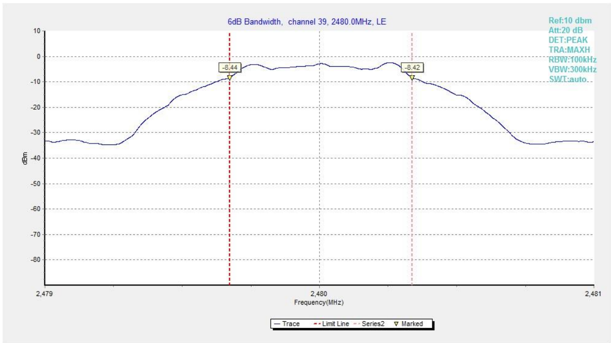
Fig.9 6dB Bandwidth (Ch 39), LE 1M
