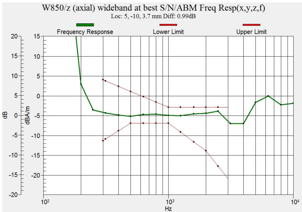
Figure B.5 Frequency Response of WCDMA Band 5
