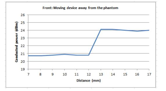
Based on the most conservative measured triggering distance of 12 mm, additional SAR measurements were required at 11 mm from the front side for the above modes.
