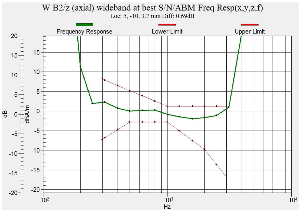
Figure B.16 Frequency Response of WCDMA Band 2 (Google Duo)
