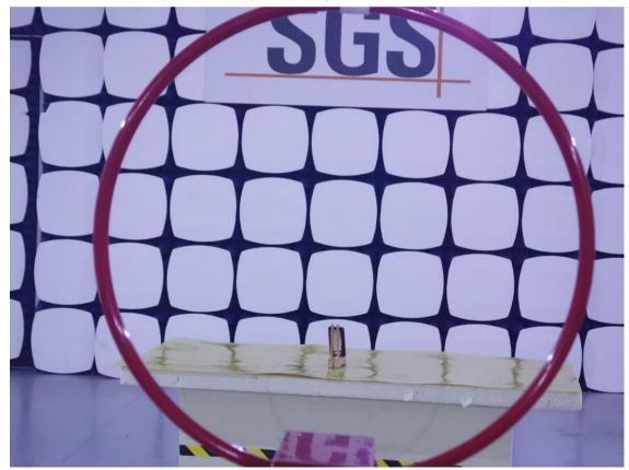
**1.3** Setup for Unwanted Emissions that fall Outside of the Restricted Bands(Radiated) and Unwanted Emissions in the Restricted Bands (Radiated) below 1GHz
