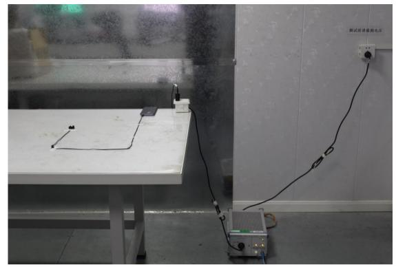
1.2 Radiated Emissions (9kHz-30MHz) Test Setup
