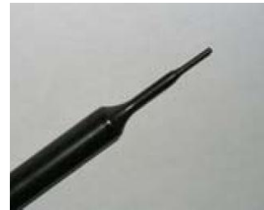
Picture C.2 Near-field Probe
