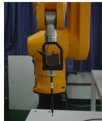
Picture C.3 E-field Probe
