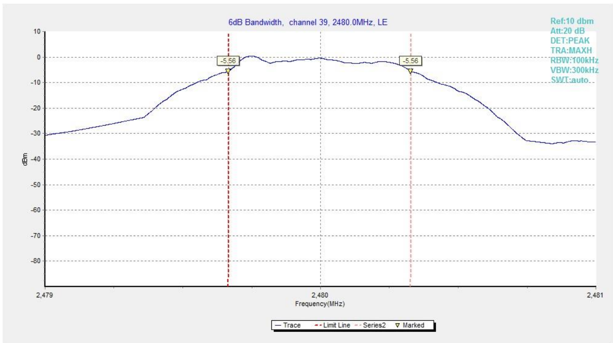
Fig.6 6dB Bandwidth (Ch 39)
