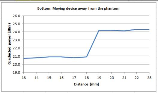
Based on the most conservative measured triggering distance of 18 mm, additional SAR measurements were required at 17 mm from the bottom side for the above modes.
