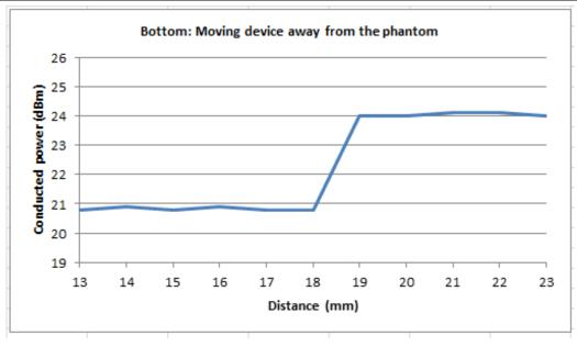
Based on the most conservative measured triggering distance of 18 mm, additional SAR measurements were required at 17 mm from the bottom side for the above modes.
