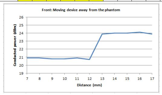
Based on the most conservative measured triggering distance of 12 mm, additional SAR measurements were required at 11 mm from the front side for the above modes.
