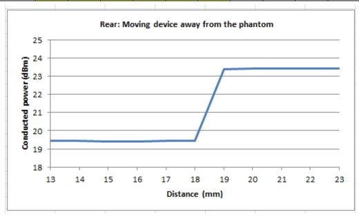
Based on the most conservative measured triggering distance of 18 mm, additional SAR measurements were required at 17 mm from the Rear side for the above modes.
