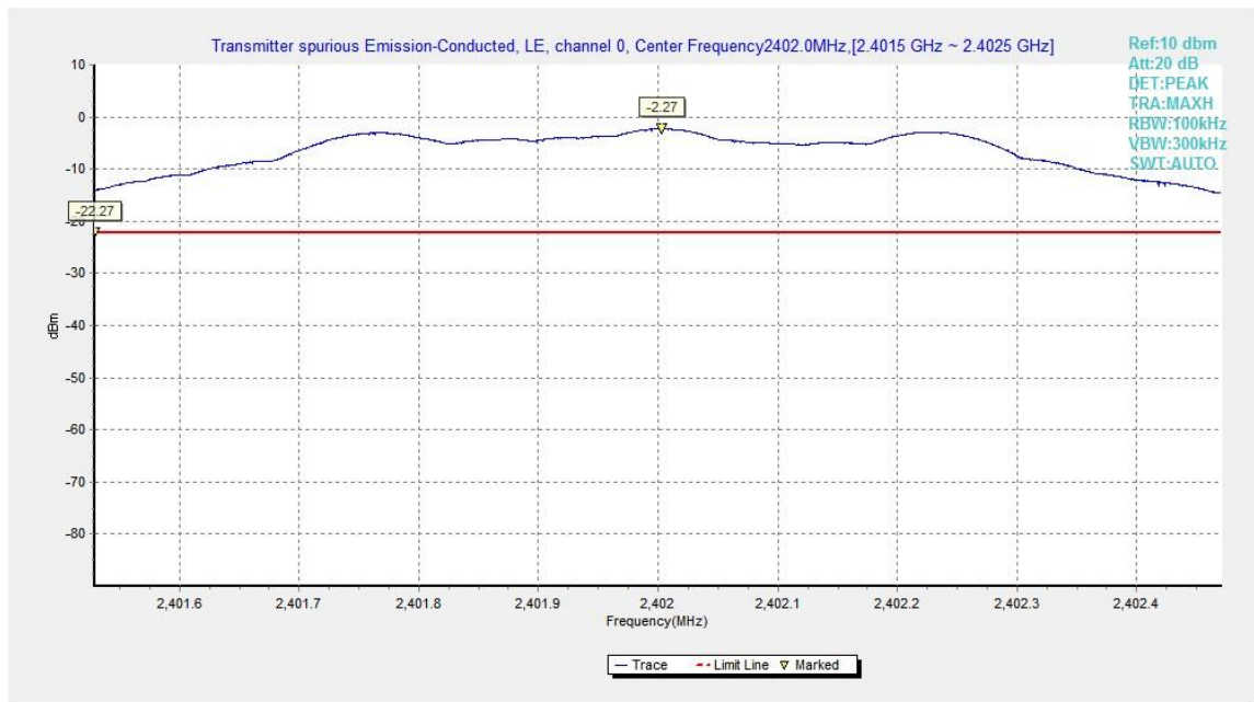
Fig.5. Transmitter Spurious Emission - Conducted: GFSK, 2402MHz
