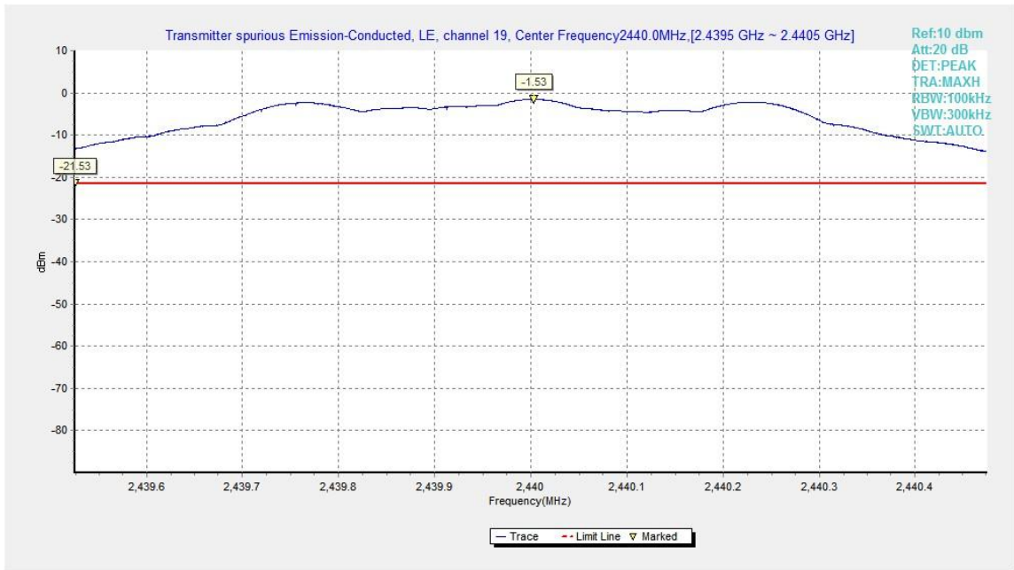
Fig.10. Transmitter Spurious Emission - Conducted: GFSK, 2440MHz
