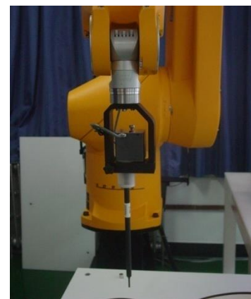
Picture C.2Near-field Probe
