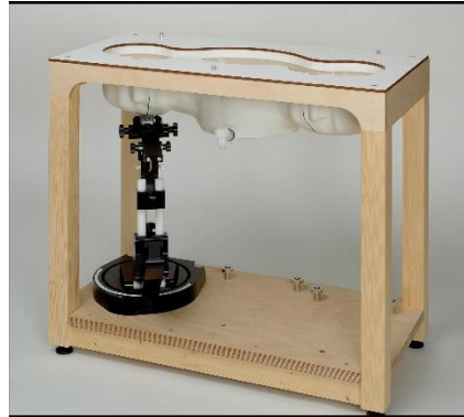
Picture C.10: SAM Twin Phantom
