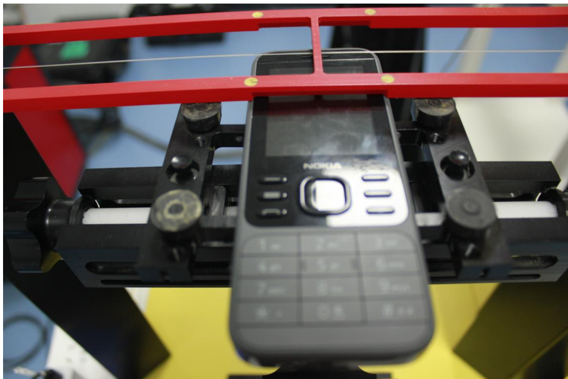
Picture 2: EUT Positioning for RF/T-coil
