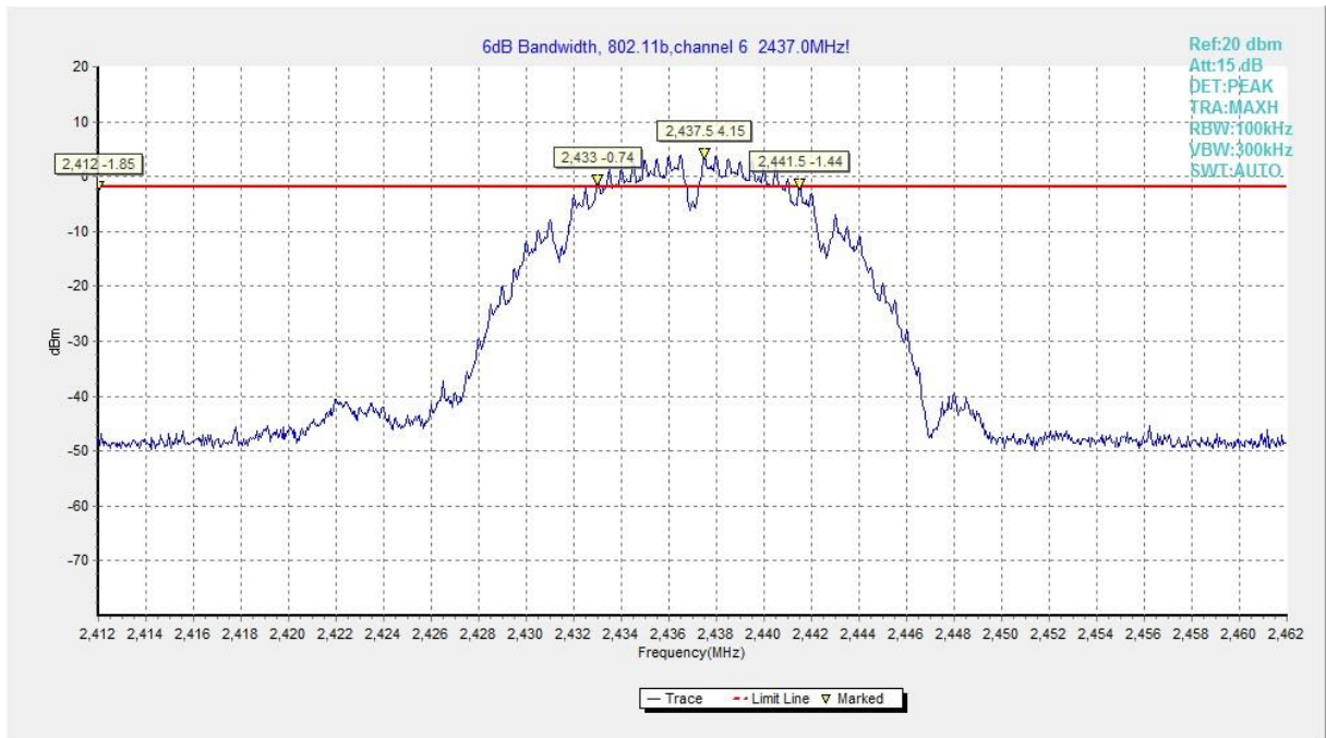
Fig.A.4.2 Occupied 6dB Bandwidth (802.11b, Ch 6)
