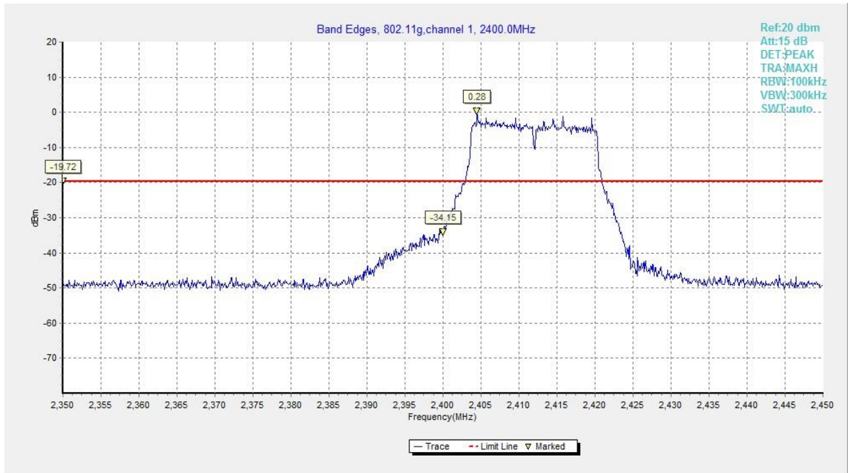
Fig.A.5.3 Band Edges (802.11g, Ch 1)
