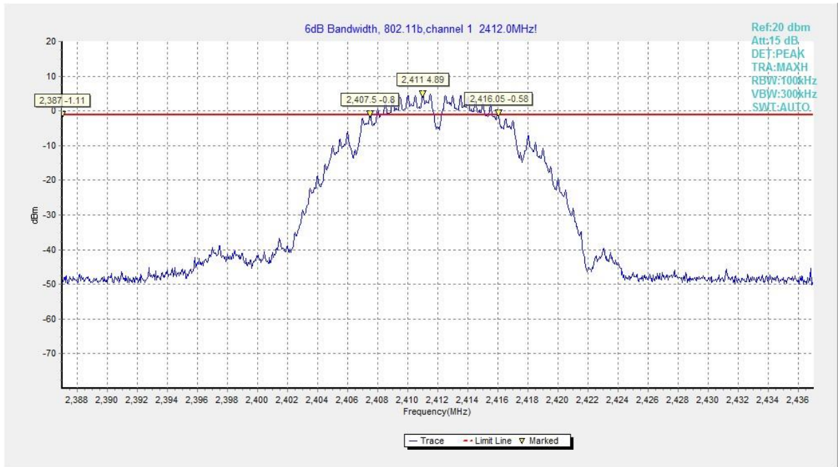
Fig.A.4.1 Occupied 6dB Bandwidth(802.11b,Ch 1)
