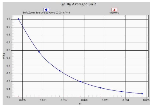
Fig. 1-6 Z-Scan at power reference point (WCDMA1900)
