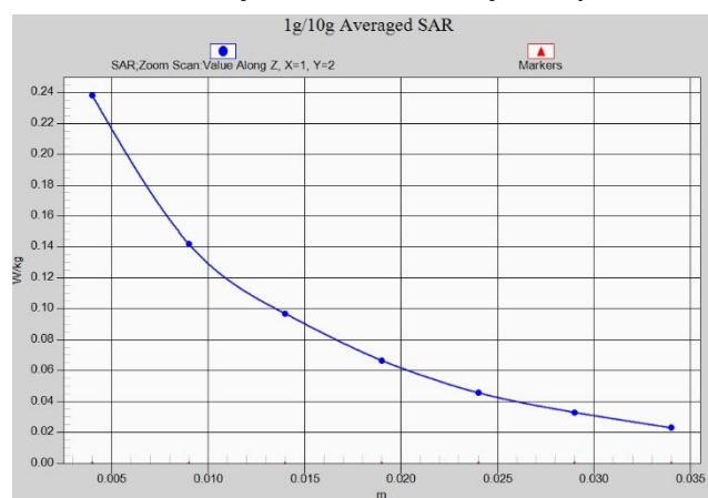
Fig. 1-8 Z-Scan at power reference point (WCDMA1700)
