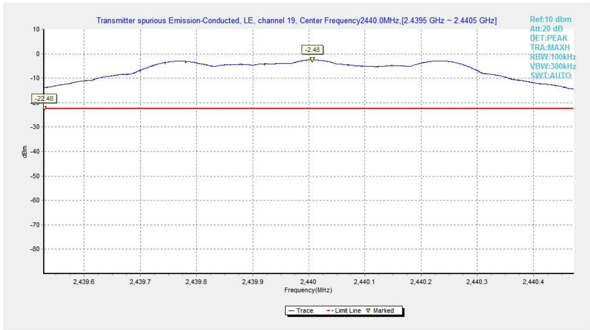
Fig.10. Transmitter Spurious Emission - Conducted: GFSK, 2440MHz
