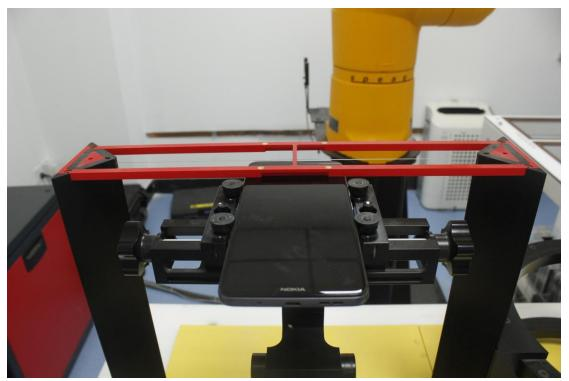
Picture 2: EUT Positioning for RF/T-coil
