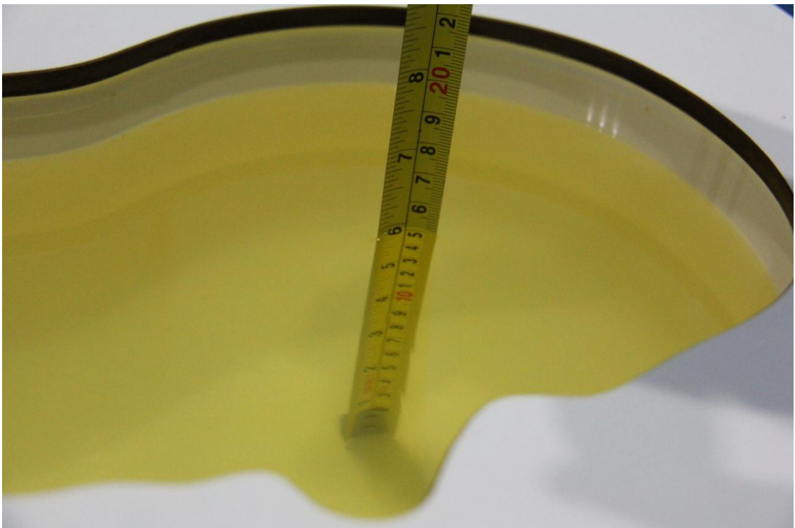
Picture 7-2 Liquid depth in the Head Phantom (1900 MHz)
