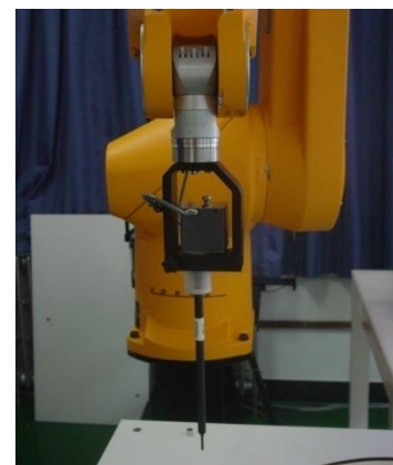
Picture C.2 Near-field Probe
