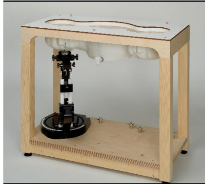
Picture C.10: SAM Twin Phantom
