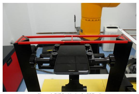
Picture 2: EUT Positioning for RF/T-coil
