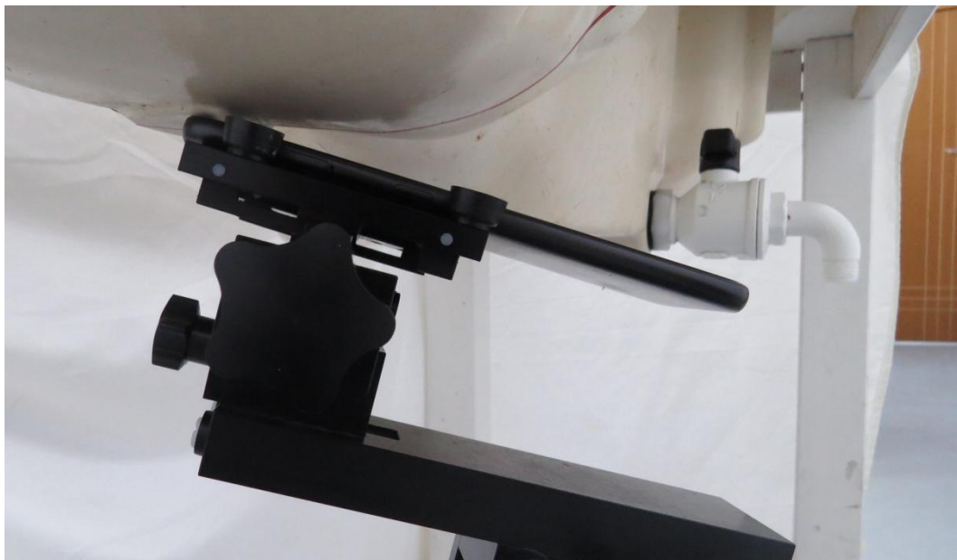
Picture 2: Right Hand Tilt 15 Degree Position
