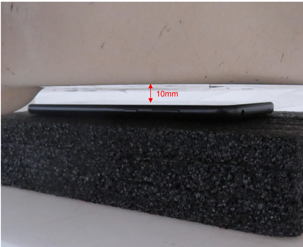
Picture 8: Front Side, the distance from handset to the bottom of the Phantom is 10mm
