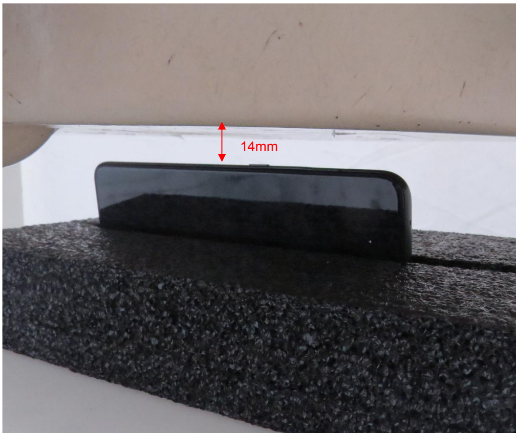
Picture 14: Left Side, the distance from handset to the bottom of the Phantom is 14mm
