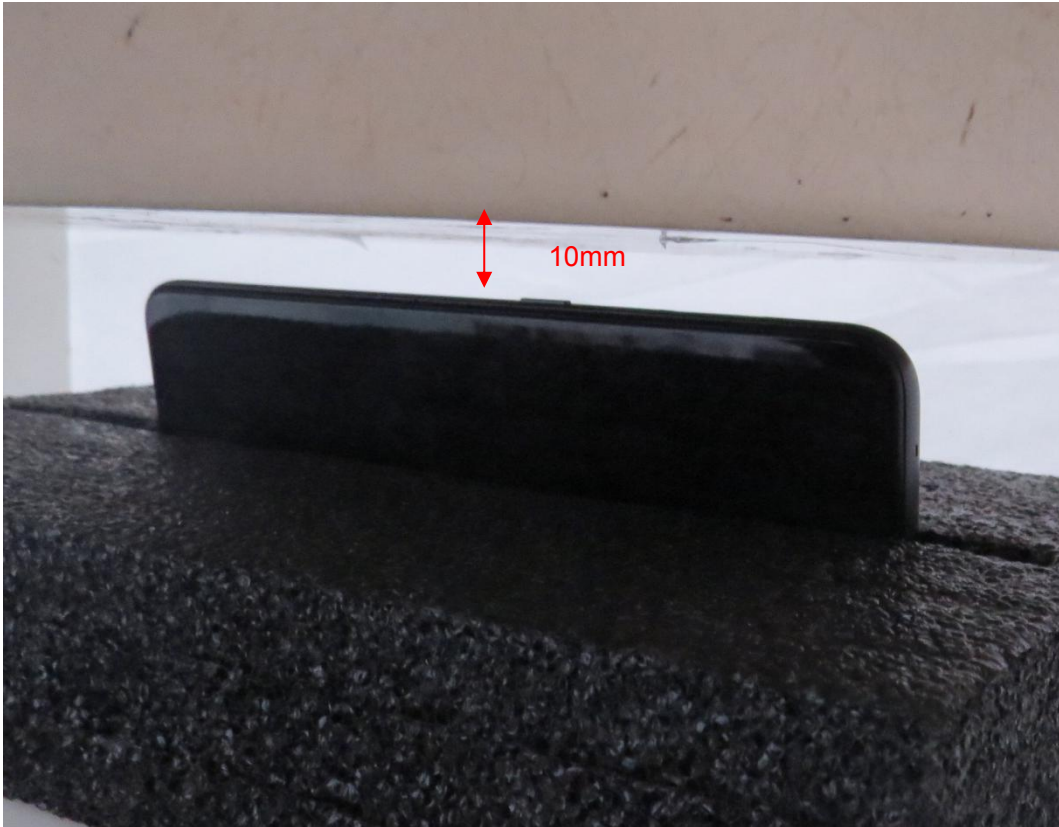
Picture 9: Left Side, the distance from handset to the bottom of the Phantom is 10mm
