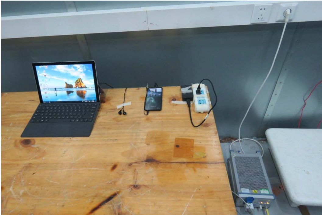
Picture 2 Conducted Emission Test Setup
