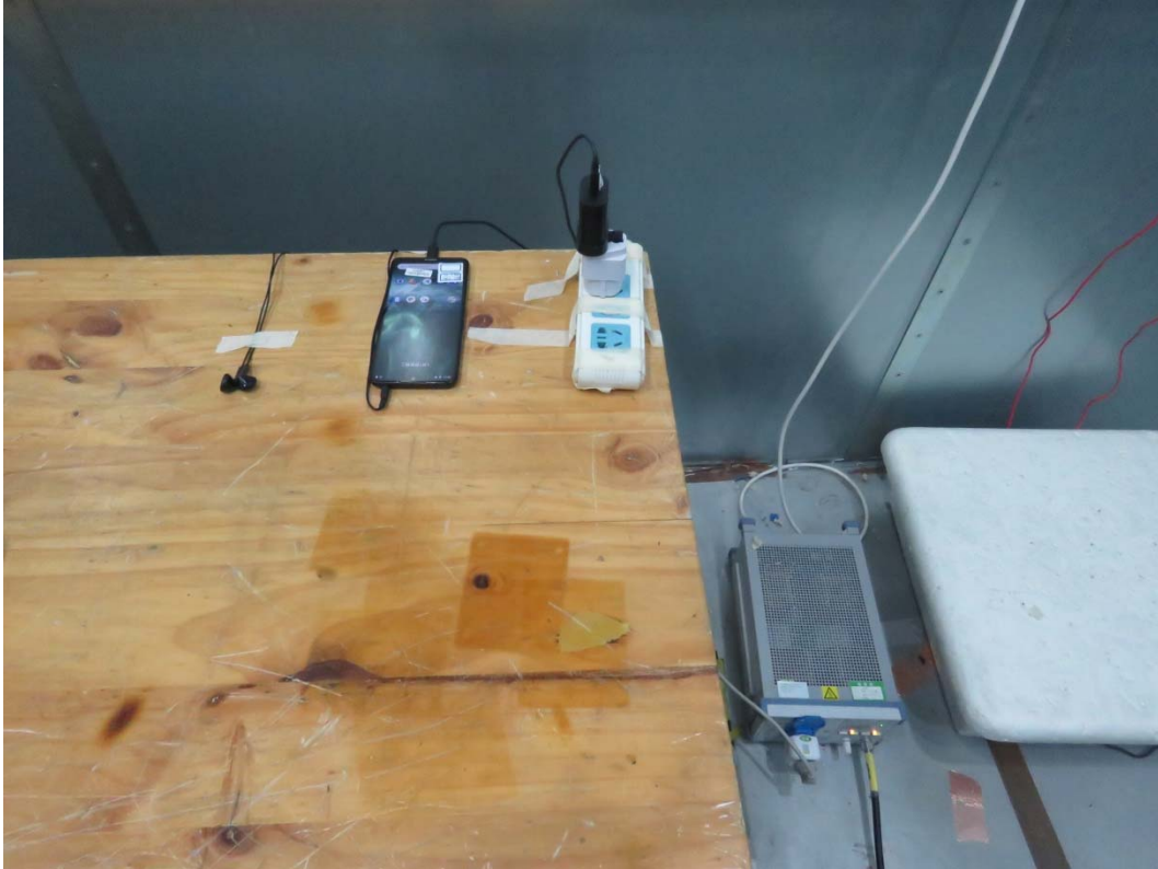
Picture 2 Conducted Emission Test Setup
