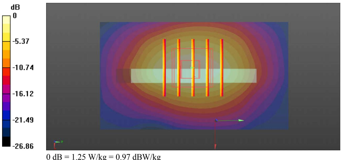
**22\_LTE Band 25\_20M\_QPSK\_1RB\_0Offset\_Bottom Side\_10mm\_Ch26140**
