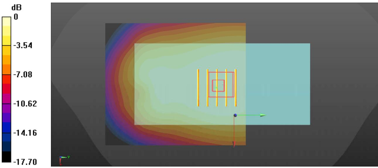
**32 LTE Band 66\_20M\_QPSK\_1RB\_0Offset\_Back\_18mm\_Ch132072**
