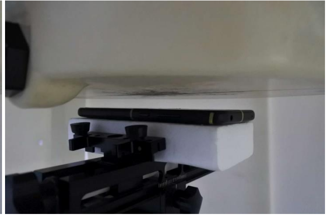
Back, Test Separation 18 mm
