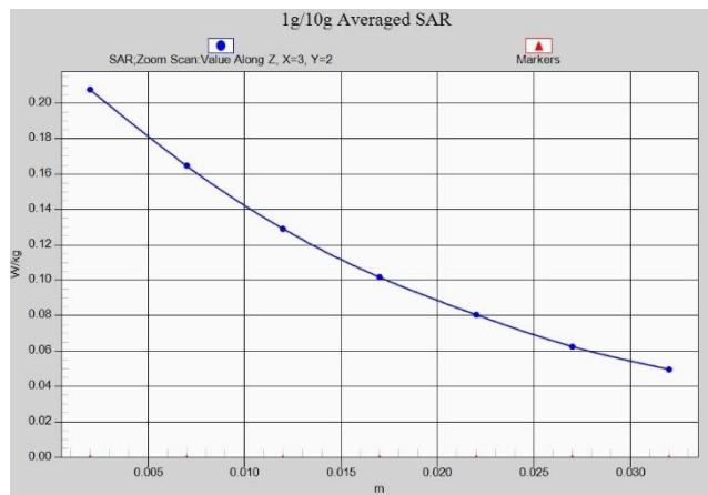
Fig. 1-1 Z-Scan at power reference point (GSM850)
