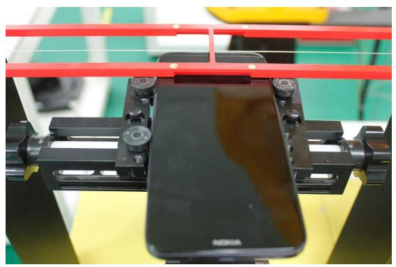
Picture 2: EUT Positioning for RF/T-coil
