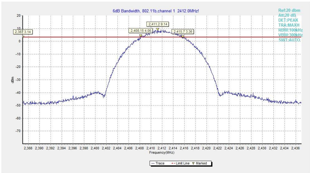
Fig.A.4.1 Occupied 6dB Bandwidth(802.11b,Ch 1)
