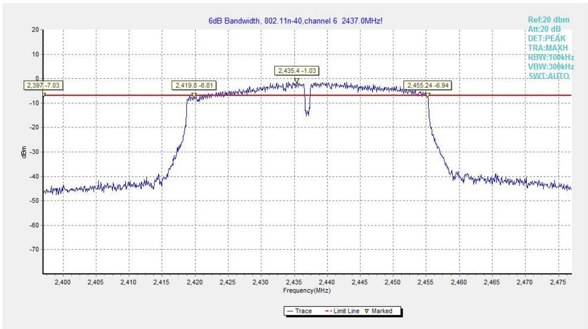
Fig.A.4.11 Occupied 6dB Bandwidth (802.11n-HT40, Ch 6)
