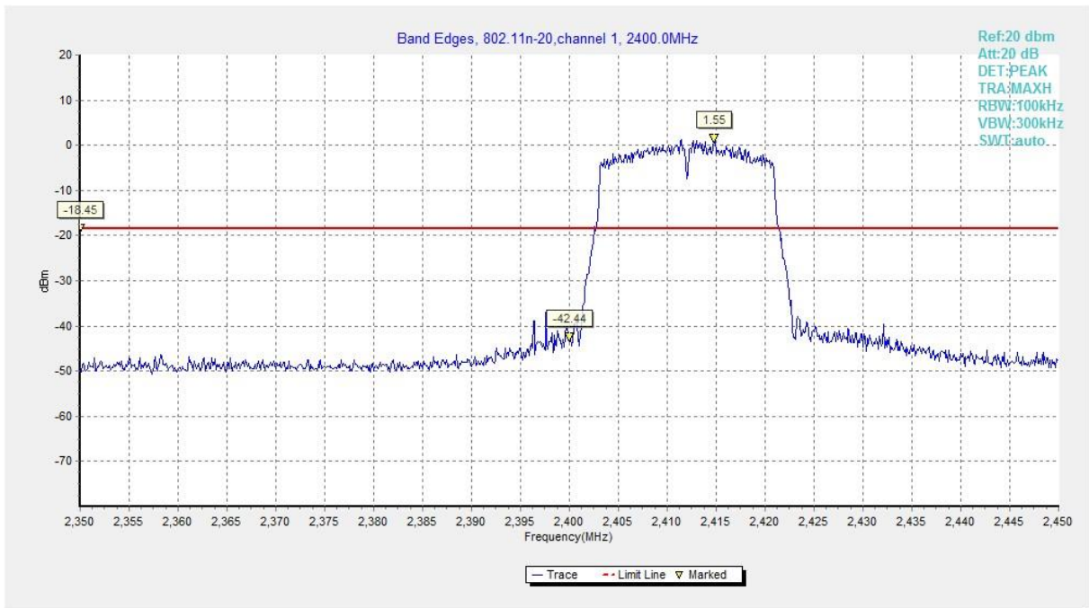
Fig.A.5.5 Band Edges (802.11n-HT20, Ch 1)
