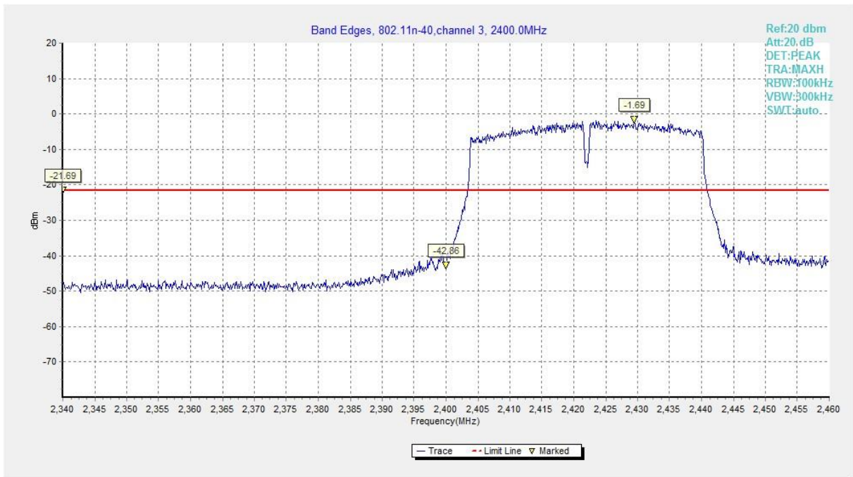
Fig.A.5.7 Band Edges (802.11n-HT40, Ch 3)
