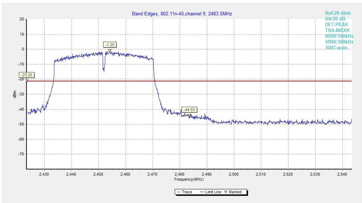
Fig.A.5.8 Band Edges (802.11n-HT40, Ch 9)
