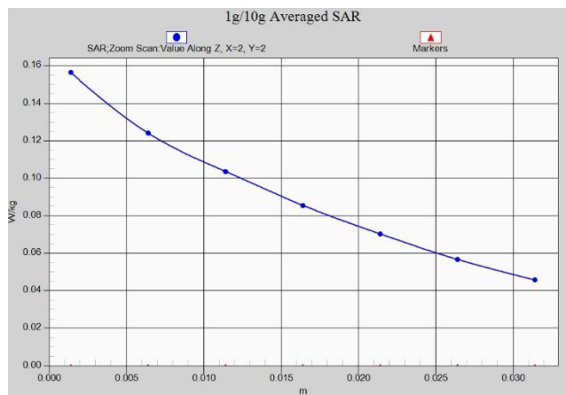
Fig. 1-17 Z-Scan at power reference point (LTE Band12)
