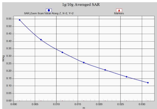
Fig. 1-14 Z-Scan at power reference point (LTE Band5)
