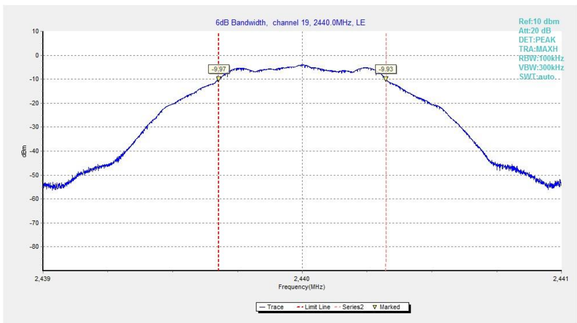
Fig.21. 6dB Bandwidth: GFSK, 2440 MHz
