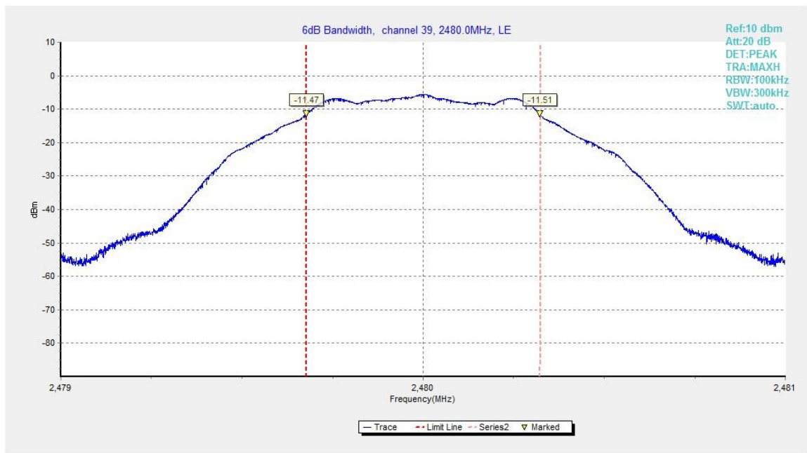
Fig.22. 6dB Bandwidth: GFSK, 2480 MHz
