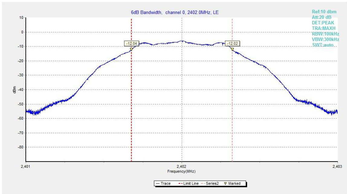
Fig.20. 6dB Bandwidth: GFSK, 2402 MHz
