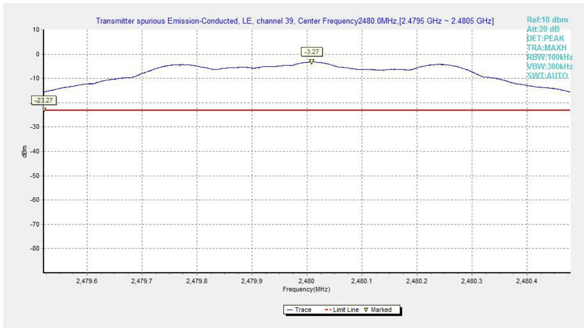
Fig.13. Transmitter Spurious Emission - Conducted: GFSK, 2480 MHz
