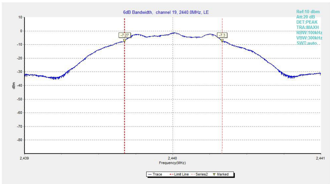
Fig.21. 6dB Bandwidth: GFSK, 2440 MHz
