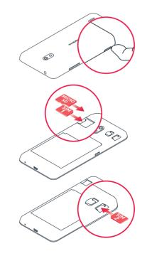
Tip: To remove the SIM card, slide the lever to the left.
