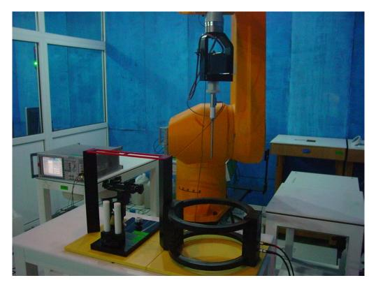
Picture A1: HAC T-Coil System Layout
