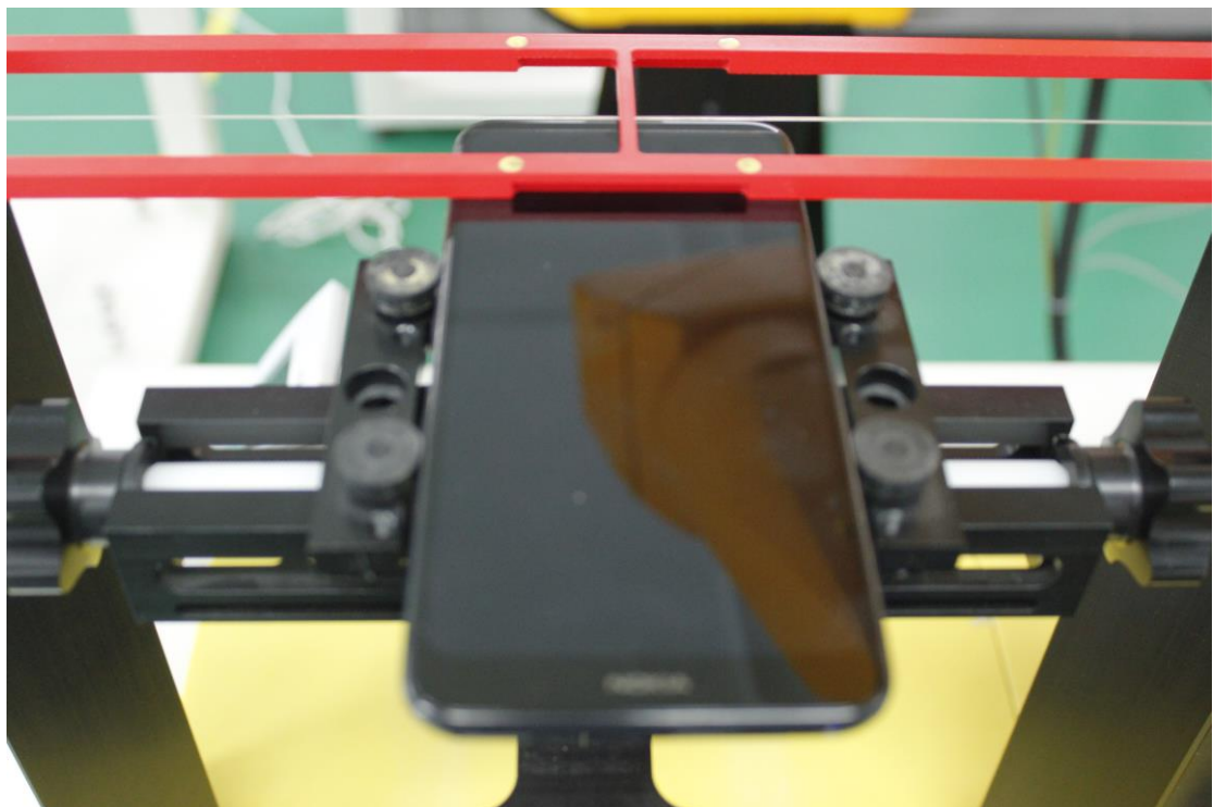
Picture 2: EUT Positioning for RF/T-coil
