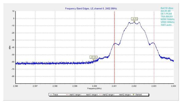
Fig.1. Frequency Band Edges: GFSK, 2402 MHz, Hopping Off
