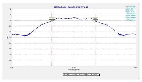
Fig.20. 6dB Bandwidth: GFSK, 2402 MHz
