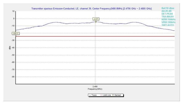
Fig.13. Transmitter Spurious Emission - Conducted: GFSK, 2480 MHz
