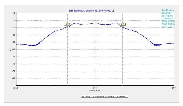
Fig.21. 6dB Bandwidth: GFSK, 2440 MHz
