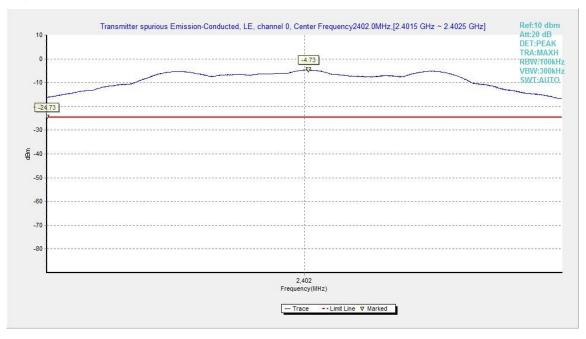
Fig.3. Transmitter Spurious Emission - Conducted: GFSK,2402MHz
