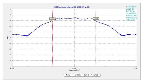
Fig.22. 6dB Bandwidth: GFSK, 2480 MHz
