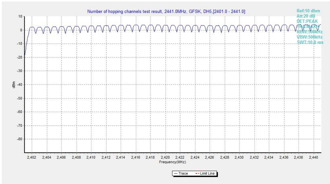
Fig.94. Number of hopping frequencies: GFSK, Channel 0 - 39
