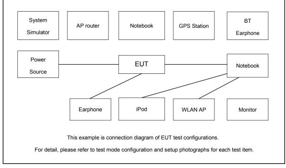
The EUT has been associated with peripherals pursuant to ANSI C63.4-2014 and configuration operated in a manner tended to maximize its emission characteristics in a typical application
