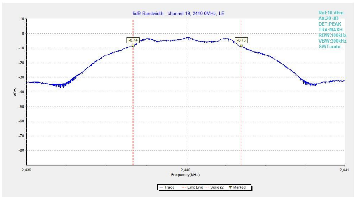
Fig.21. 6dB Bandwidth: GFSK, 2440 MHz
