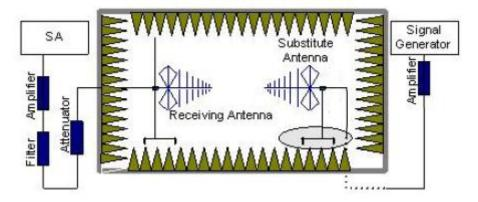
In the chamber, an substitution antenna for the frequency band of interest is placed at the reference point of the chamber. An RF Signal source for the frequency band of interest is connected to the substitution antenna with a cable that has been constructed to not interfere with the radiation pattern of the antenna. A power  $(P_{Mea})$  is applied to the input of the substitution antenna, and adjusts the level of the signal generator output until the value of the
