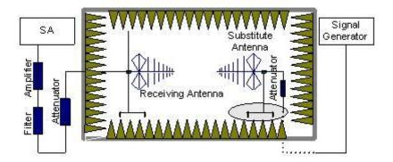
In the chamber, an substitution antenna for the frequency band of interest is placed at the reference point of the chamber. An RF Signal source for the frequency band of interest is connected to the substitution antenna with a cable that has been constructed to not interfere with the radiation pattern of the antenna. A power ( $P_{Mea}$ ) is applied to the input of the substitution antenna, and adjust the level of thesignal generator output until the value of the
