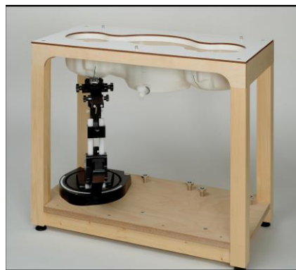
Picture C.10: SAM Twin Phantom
